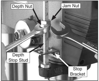
Figure 29. Depth stop components.
